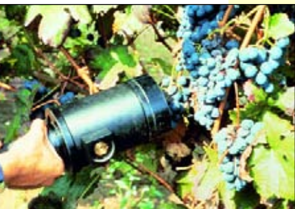
Collecting samples of Botrytis cinerea from grapes by a battery-driven, portable spore-trapping device. A vacuum deposits spores on a fungicide containing agar plate. (M.L.Gullino, University of Turin)
